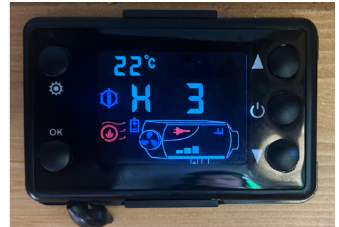
Running On Fan Speed
