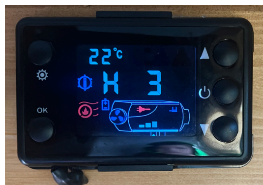
Step 2: The mountain symbol should've disappeared. This can be done with the heater on or off.
