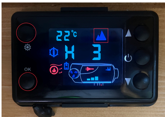
Step 1: Hold the "Settings Button" and "Ok Button" simultaneously until the mountain symbol has disappeared.
